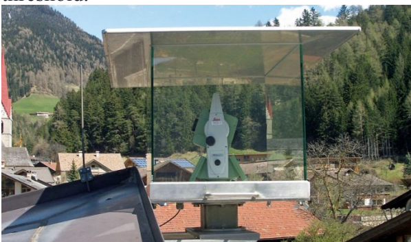
Fig. 4 Mountainous area monitoring using total station
