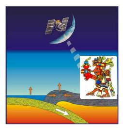
Interaction between the subducting oceanic and overriding continental plates produces a surface crustal deformation which can be measured and monitored by permanent GPS stations.
