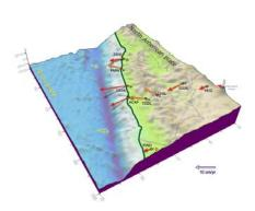
2001-2002 Silent Earthquake (red vectors) was the largest one (Mw ~ 7.5) ever recorded with GPS. Yellow vectors show interseismic steady state GPS stations velocities.
