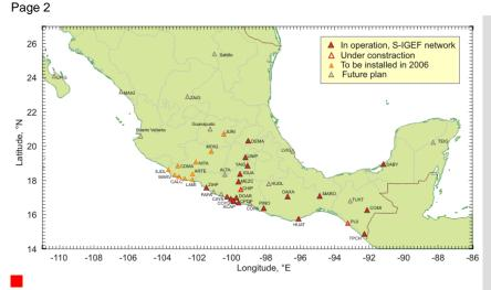
Permanent GPS network Sismologia-UNAM accounts for 19 stations (15 stations are equipped with Leica GRX1200 and SR500 receivers and AT504 antenas). Ten more RGX1200 receivers will be installed in 2006.
